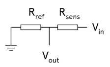
A voltage divider configuration is the simplest readout circuit to determine sensor resistance. Given that  $R_{ref}$  and  $V_{in}$  are known, the sensor resistance  $R_{sens}$  can be calculated by measuring the voltage drop  $V_{out}$  across the reference resistor  $R_{ref}$ .
